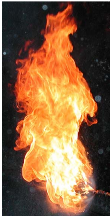
Figure 2. A typical hydraulic oil spray flame
